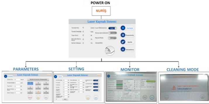
Figure 16 Laser Welding System Main Screen
