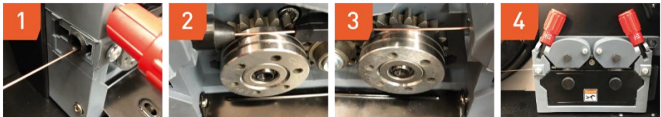
Figure 3.8 Welding wire connection
